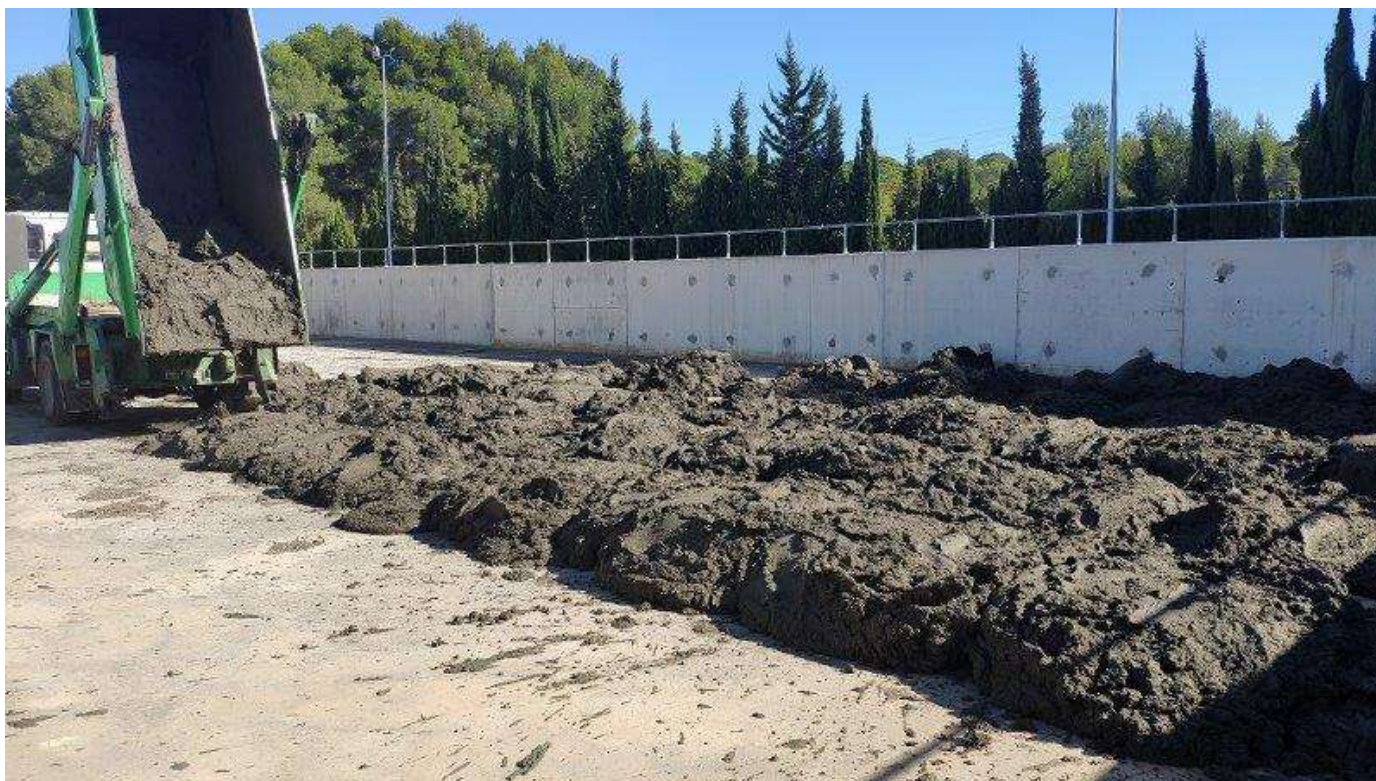
Figure 1. DWTS open-air solar drying before granulation process.
