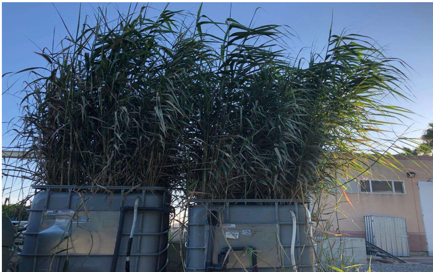
Figure 2. VFCW pilot plants with DWTS as substrate active.
